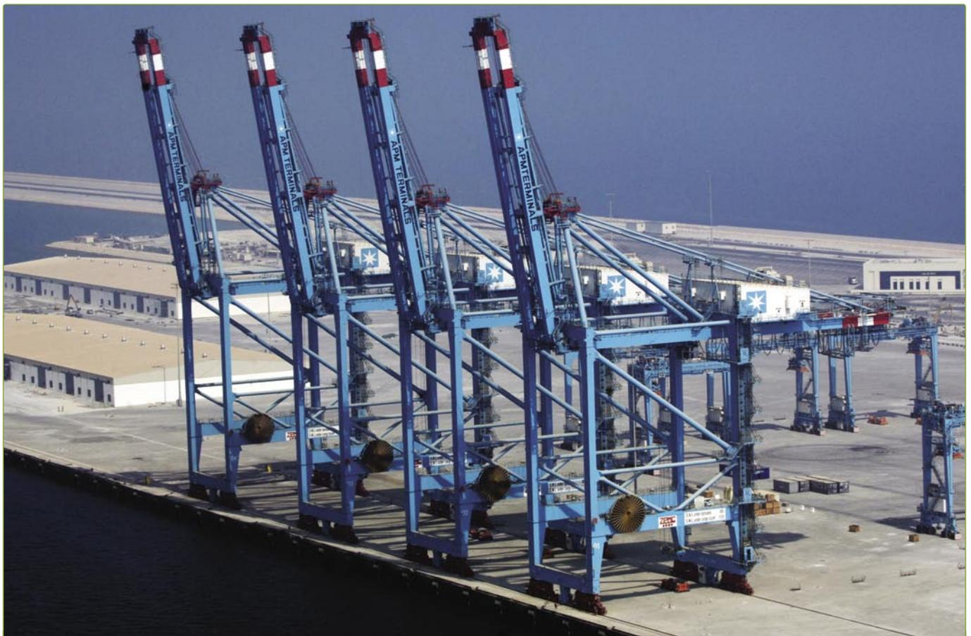
Figure 1. The port is equipped with four new Post Panamax cranes, each fitted with twin spreaders.
